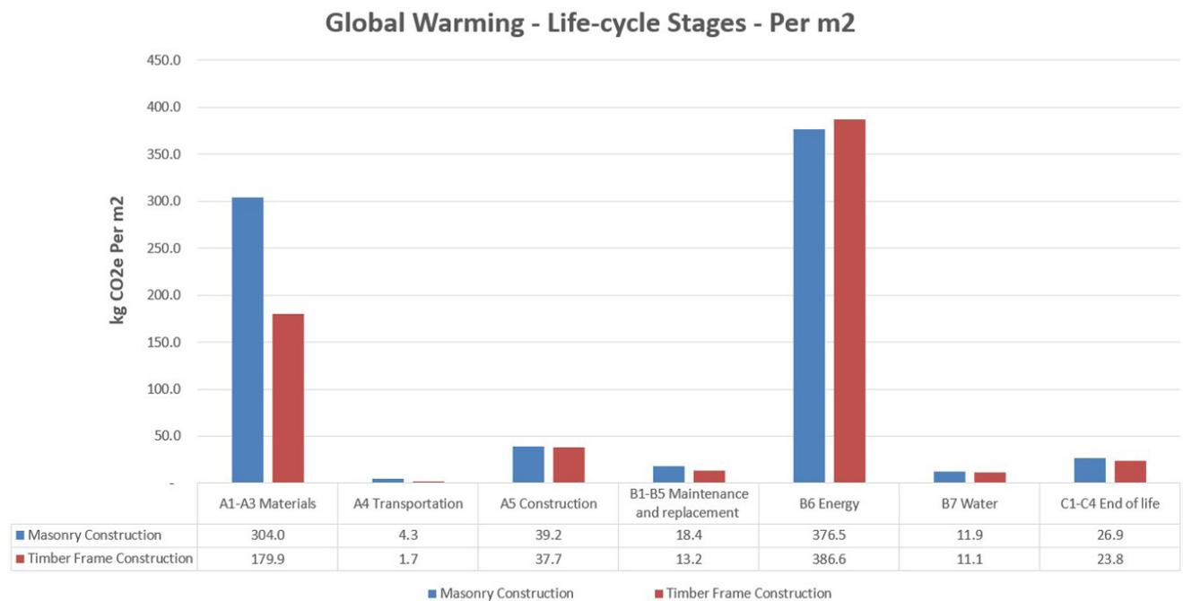
**Figure 19.** Life-Cycle Stages Comparison
