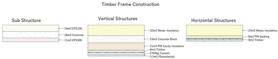
Figure 12. Timber Frame Construction Main Materials
