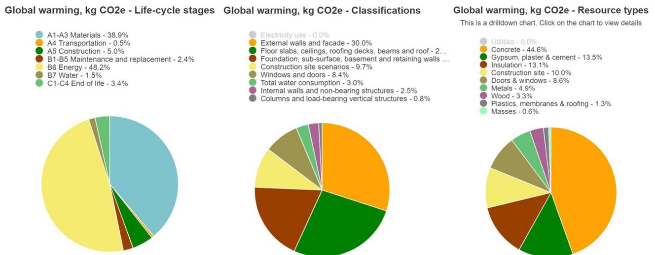
Figure 14. Masonry Construction Global Warming - Life-Cycle Stages, Classifications, Resource Types
