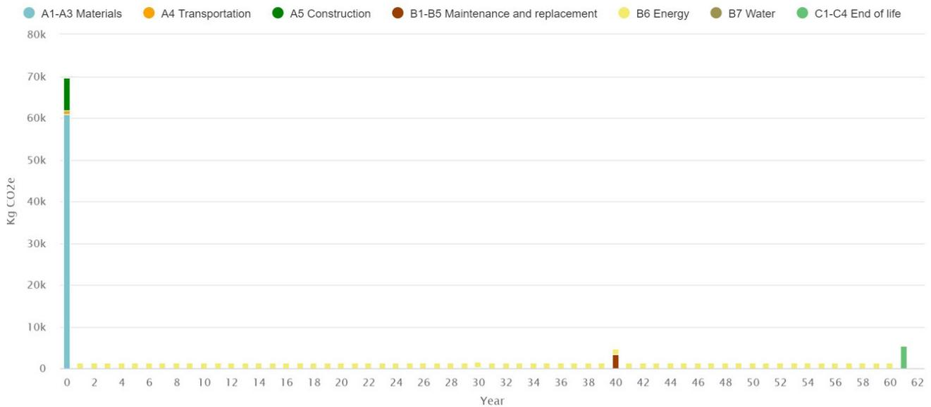
Figure 15. Masonry Construction Annual Impacts
